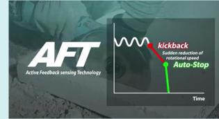
Active Feedback sensors (AFT), mechanical brake, anti-restart, and soft start.
