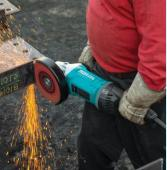
Anti-vibration housing and vibration proof grip minimise user fatigue.
